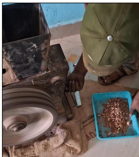
Fig 9.3: Jaw crushed samples prepared for pulverizing
