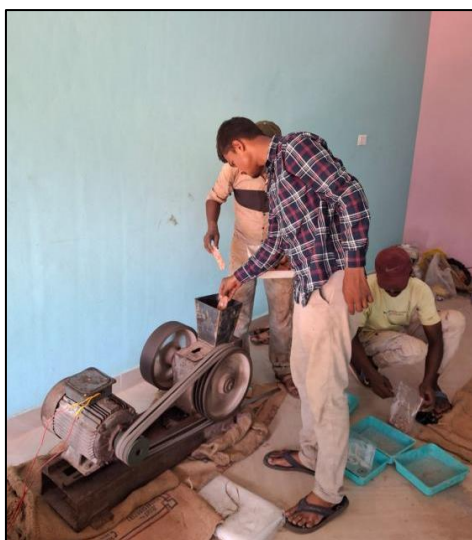
Fig 9.2: Cut split cores introduced Jaw crusher
